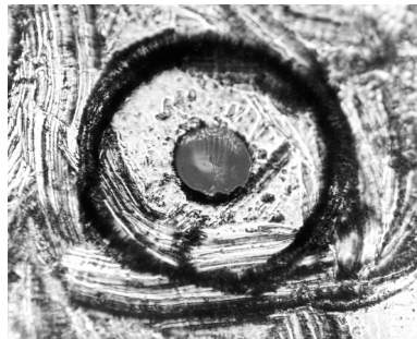
Figure 5-6. Damage from improper cleaning.
